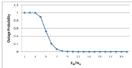
**Figure 6:** Outage Probability of QPSK for nakagami-n channel model for various values of  $E_b/N_0$  taking  $n=7$  and  $\gamma_{th}=5$
