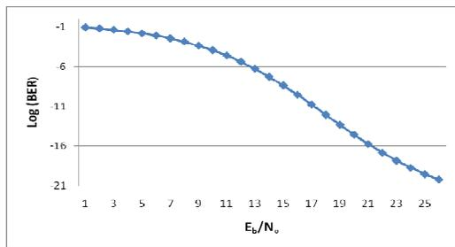
**Figure 5:** Bit Error Rate of QPSK for Nakagami-n channel model for various values of  $E_b/N_0$  taking  $n=7$
