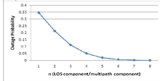
**Figure 7:** Outage probability of QPSK for various values of Nakagami-n channel model parameter ‘ $n$ ’ taking  $\gamma_{th}=5$  and avg.  $E_b/N_0=15$ .
