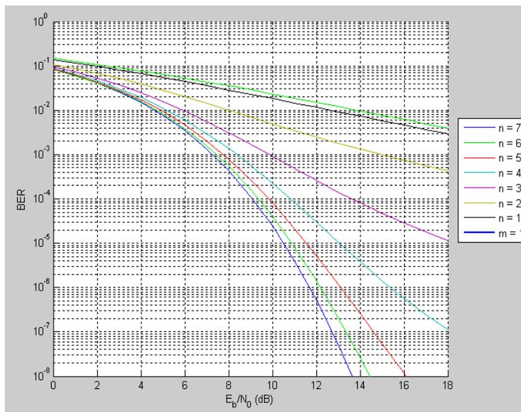
**Figure 8:** BER of QPSK for various values of  $n$  (Nakagami- $n$  parameter) and for  $m=1$  (Nakagami- $m$  parameter)
