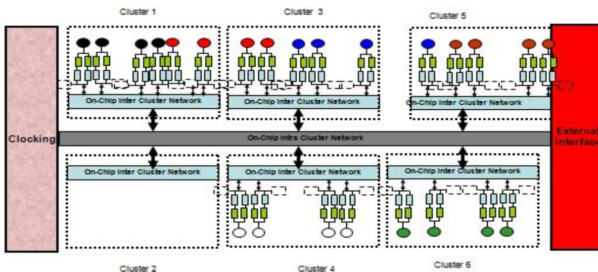
Fig. 1: Architecture of HMPM showing implementation of Processing-Stealing Technique after subjecting to workloads of 6:5:5:0:4:4 reconfiguration ratios
