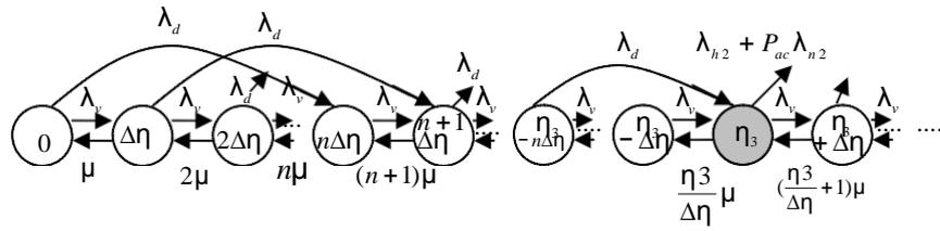
**Figure 2:** Multitransition  $M/M/\eta_{\max}/\eta_{\max}$  loss Markov model
