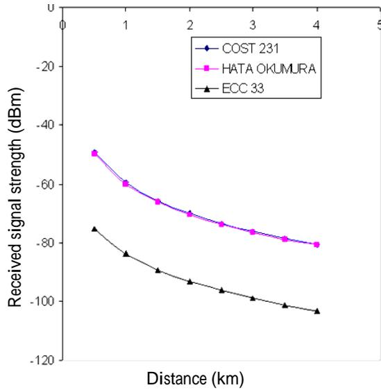
Fig.3 Received signal strength for suburban models
