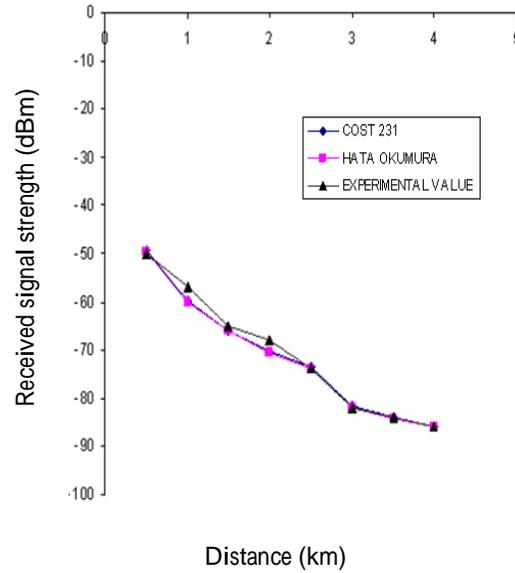
Fig. 4 Received signal strength for highway models
