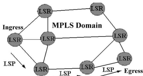
Figure 2: A typical MPLS domain with edge routers
