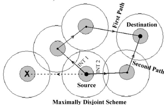
**Figure 6:** Multipath Routing Scheme in AODV
