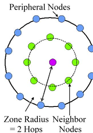
Figure 14: Three types of Nodes in ZRP
