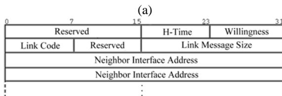
**Figure 11:** OLSR Packet Format (a) and Hello Format (b)
