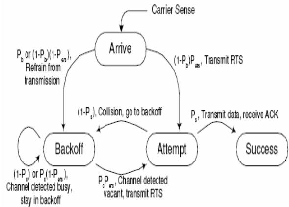
**Figure 6:** Transmission energy consumption model for nanoMAC.
