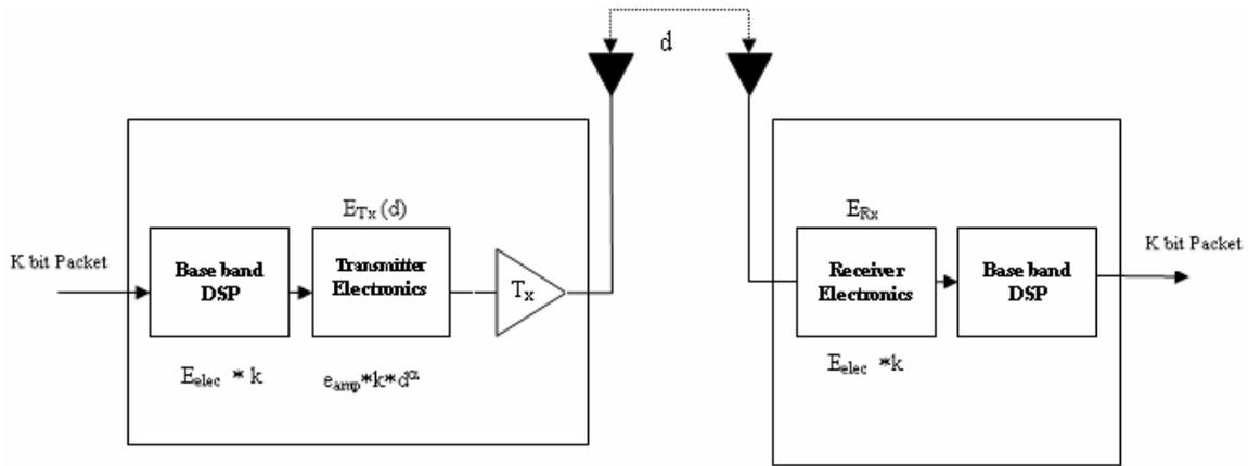
**Figure 1:** Energy consumption model for communications.
