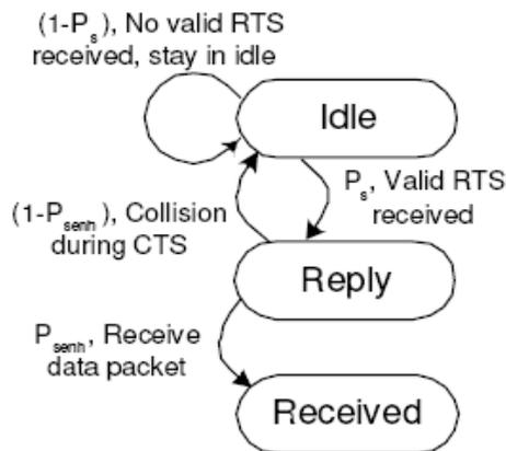
**Figure 7:** Receive energy consumption model for nanoMAC.
