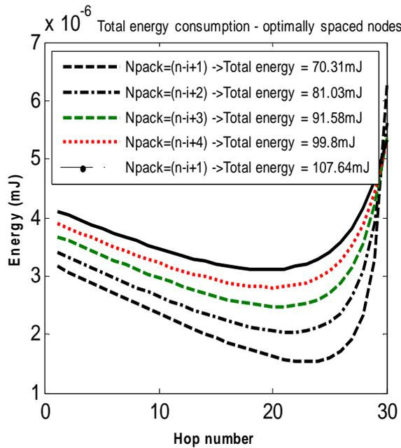
**Figure 5:** Energy consumed with optimal transmission distances.
