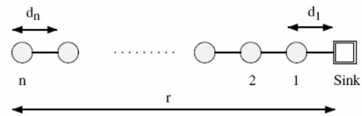
**Figure 2:** Multi-jump linear model featuring equal distances between the nodes.
