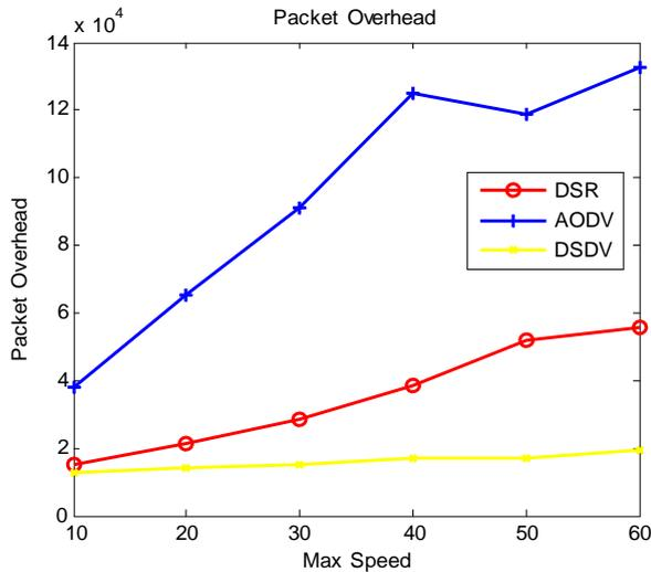
Figure7.control packet overhead
