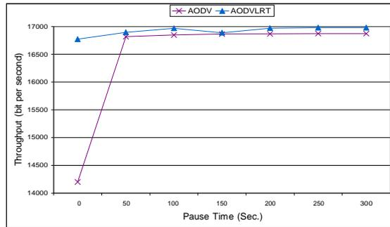
**Figure 3:** Throughput vs. pause time for 50 nodes
