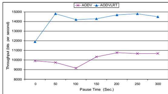
Figure 6: Throughput vs. pause time for 100 nodes
