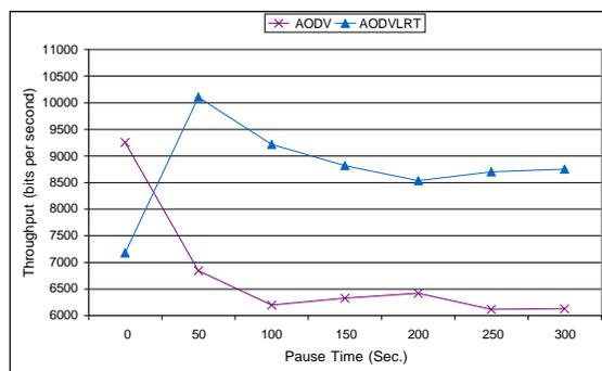
**Figure 9:** Throughput vs. pause time for 300 nodes
